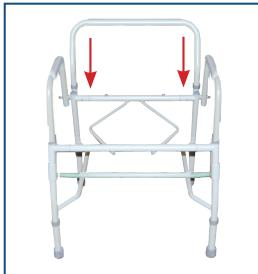
4. Align the toilet seat clamps onto the back frame rail. (Both clamps should sit outside the pail brackets). Push down on seat until clamps snap firmly into place. Repeat for the lid. To remove, grasp the back of the seat and lift.
