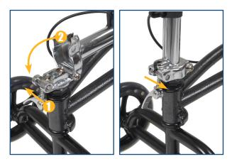
3. Slide locking mechanism into groove on tiller, depress locking handle to secure tiller lock.
