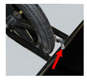
Now set the removed nut aside while you slip the splash guard onto the caliper mounting bolt. Hold the splash guard in place and reinstall the mounting nut.
