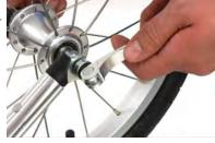
standard front wheel by unfolding the quick release lever and sliding the wheel out of the fork tips. Next loosen the black knob on the top of the Axis swivel wheel adaptor and unfold the hinged lid.
