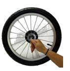
Next, push the black button and while holding it in... ...insert the wheel axle all the way into the pushchair frame and release the button.
