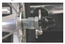
Position the silver lever straight out from the frame as shown. Now tighten the black knob on
