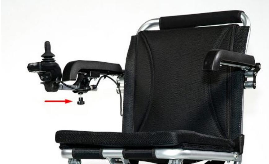
**Manual-Electric drive conversion** Lock the brake and turn off the power; pull the clutch (with red switch) out of the slot and turn right or left, make sure the clutch will not fall into the slot it is manual drive mode. Pull and turn the clutch again and make the clutch fall into the slot. It is electric drive mode.
