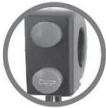
**(top) Red button** : pressing the red button will put the EzFold scooter in reverse mode
