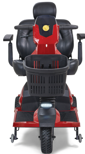
Front and rear LED lights and side reflectors for safety
