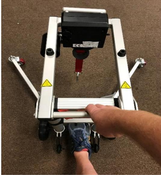
5) Raise the telescoping poles, place your foot on the black bar between the two anti-tip wheels (as shown in the photo to the left). Then lift up on the handle (as also shown in the photo to the left). Raise to the desired height.
