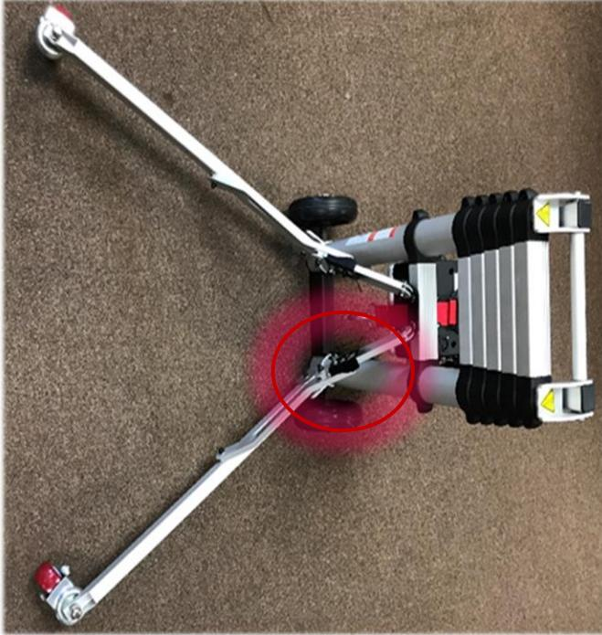
3) Make sure the hinge (located in red circle on the photo to the left) is locked before moving to the next step.
