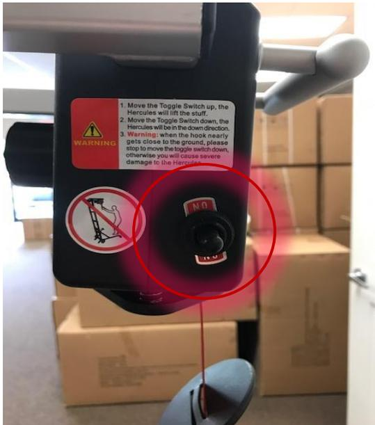
8) Lower the belt to desired length by pressing the dual switch on the motor of the scooter lift down towards the ground (as shown in the photo to the left in the red circle).
