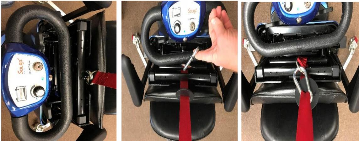
**10) To raise the scooter off the ground, make sure the brake is engaged and push up on the dual switch located on the motor of the scooter lift. See Photo below**
