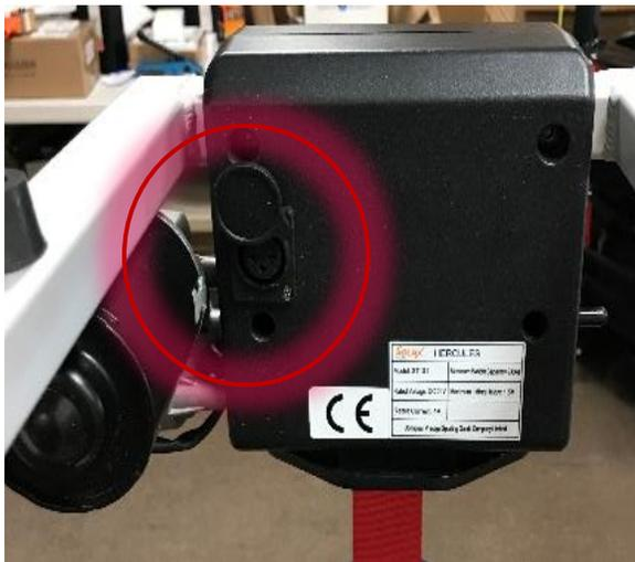
7) Attach the other end of the power cord to the port on the Hercules Lift Motor (as shown in the red circle in the photo to the left).
