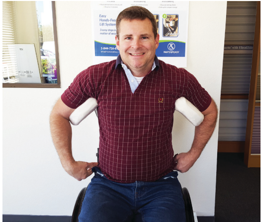
Figure 2: While in use Pads rotate approximately 45 degrees to complete the lift motion.
