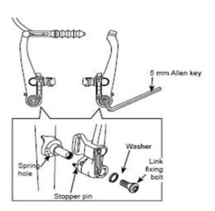
2. While holding the shoe against the rim, adjust the amount of shoe protrusion by interchanging the position of the B washers (i.e. 6 mm and 3 mm) so that dimension A is kept at 39 mm or more.
