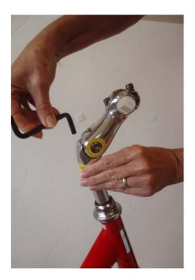
c) Loosen the 2 hex head screws located on the top of stem and remove handlebar clamp. Place the handlebars on the stem and replace the handlebar clamp.
