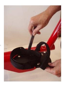
b) Pedals adjust to size. Length can be shortened or lengthened to fit foot. Position of pedal over axle can also be adjusted. Use the quick release wrench slotted end to easily loosen and tighten wing nuts.
