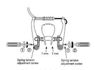
4. Pass the inner cable through the inner cable lead. Set the cable with the clearance of 1mm between each brake pad and the rim, tighten the cable fixing bolt.
