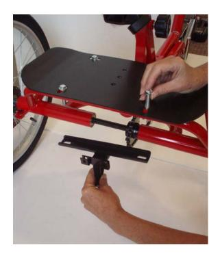
c) Mount basket into slots in bracket. Use the optional screws if basket is permanent attachment.
