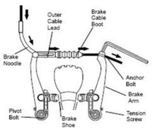
6. Depress the brake lever about 10 times as far as the grip to check that everything is operating correctly and that the shoe clearance is correct before using the brakes.
