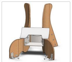
Attach (D) front brackets to (A) wooden sides with (4x) bolts. Finger tighten bolts first, then securely tighten with wrench.
