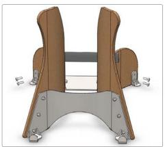
Attach (D) front brackets to (A) wooden sides with (4x) bolts. Finger tighten bolts first, then securely tighten with wrench.
