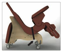
Secure tightly the Bottom Strap under Mobile Floor Base.
