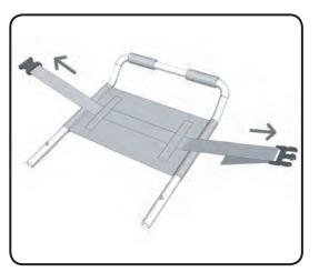
To attach the chest belt rotate the chair so that you have easy access to the back of the back rest.
