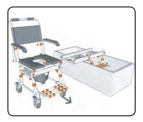
Ensure the primary brake securely locks your Showerbuddy SB2 in position on the wheeled base before disconnecting the bridge.
