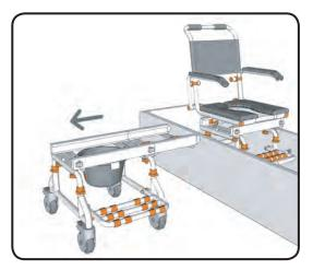
With your Showerbudd SB2 secured in position on the bath base remove the bridge and wheeled base.
