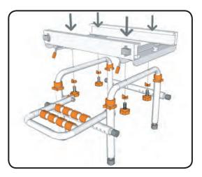
Using the grooves on the underside of the bath base track as a guide, place the bath base track onto the height adjustment tubes.
