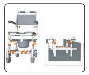
The wheeled base, bridge and bath base should now be securely connected together using the latches.
