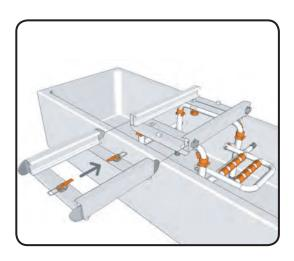
Align the bridge with the bath base and insert the tongues into the bath base.
