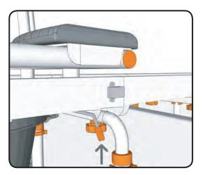
To transfer your Showerbuddy SB2 back to the wheeled base lift and hold the primary brake lever to release the chair. The The primary brakes are located on each side of the wheeled and bath base tracks at the front.
