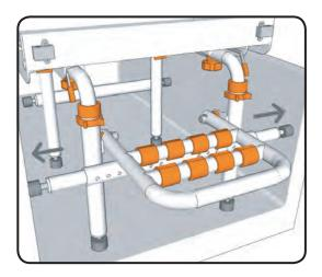
With the bath base placed in the bath secure it in position by adjusting the stabilising tubes.
