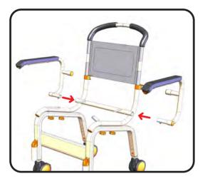
Fit Left Hand Arm (part #500-043) and Right Hand Arm (part #500-045) by positioning the axle (smaller diameter) part of the tube against the hollow tube across the rear of the Seat Frame (part #500-021) and sliding into this tube.
