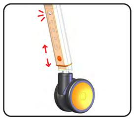
To adjust the Seat Height adjust the Caster Legs (part #500-296 front & 500-010 rear) by using the Push Pins in the legs and ensure that the push pins fully engage the height adjustment holes evenly.
