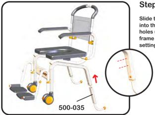
Slide the anti-tip leg (part# 500-035) into the frame as shown. Line the bolt holes up with the desired holes in the frame for your chosen chair height settina.
