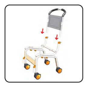
Slide Back Rest Frame (part #500-042) down through Arm Clips (part #500-237) and into the Seat Frame (part #500-021). Make sure that push pins are fully depressed before inserting the back rest frame.
