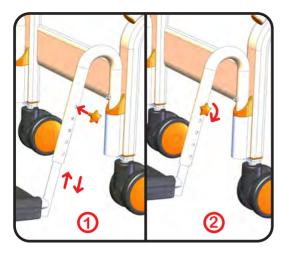
Adjust the Footrest height to suit the user as shown ensuring that the screw lock is fully tightened and the foot supports are level.
