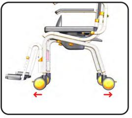
The caster wheels should be rotated outwards towards the front and rear of the chair to make the chair more stable during transfers.
