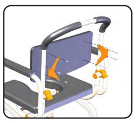
To install, simply remove the safety restraint clamp bars (part #500-106) and replace them with the two back rest support arms shown.
