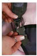
Push down on the silver center button located between the passengers knees and pull the webbing out to the end.
