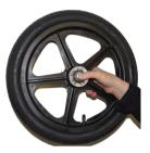
Next, push the black button and while holding it in... ...insert the wheel axle all the way into the pushchair frame and release the button.
