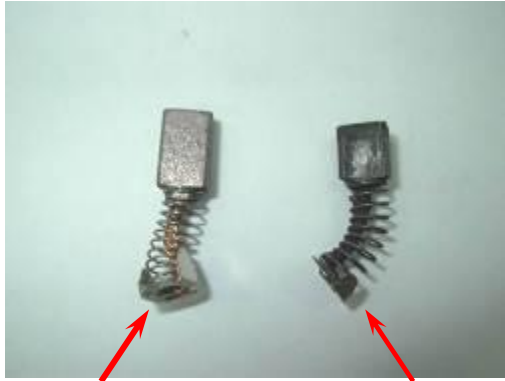
New Motor Brush Worn Motor Brush (Fig 26)
