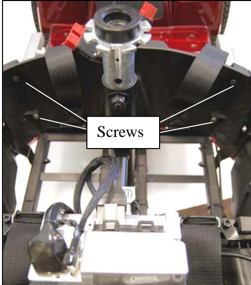
Figure 16. Inside Battery Compartment
