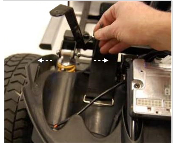
Figure 24. Shock Bolt Removal
