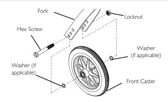
FIGURE 7 Replacing Front Casters
