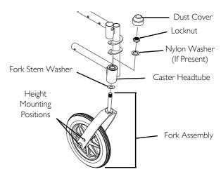
FIGURE 6 Installing/Replacing Front Casters and Forks
