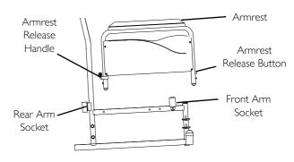
FIGURE 6 Removing/Installing Armrests
