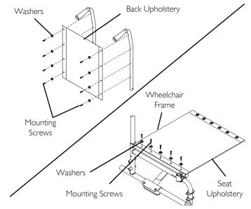
FIGURE 2 Replacing Back Upholstery/Replacing Seat Upholstery
