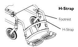
FIGURE 8 Installing H-Strap/Calf Strap
