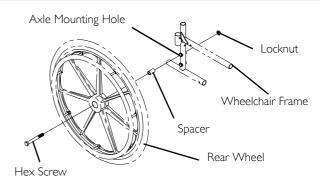
FIGURE 4 Removing/Installing Rear Wheels
