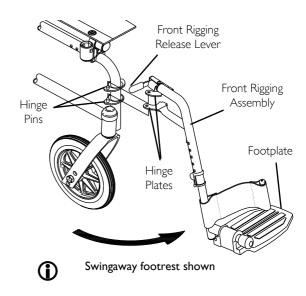
FIGURE 4 Installing/Removing Front Riggings
