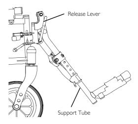
FIGURE 5 Raising/Lowering Elevating Legrest Assembly
