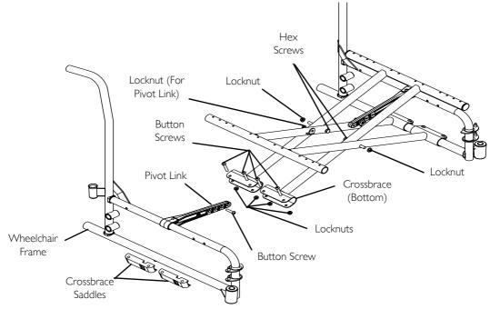
FIGURE 3 Adjusting the Seat Width
