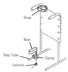
FIGURE 2 Installing Crutch and Cane Carrier
