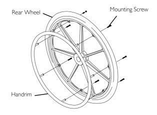
FIGURE 5 Replacing Rear Wheel Handrim
