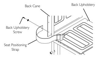
FIGURE 3 Installing the Seat Positioning Strap
