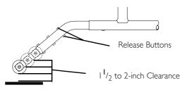
**FIGURE 5** Adjusting the Anti-Tippers
