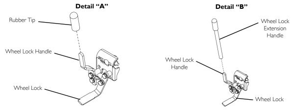
FIGURE 9 Installing the Optional Wheel Lock Extension Handle
