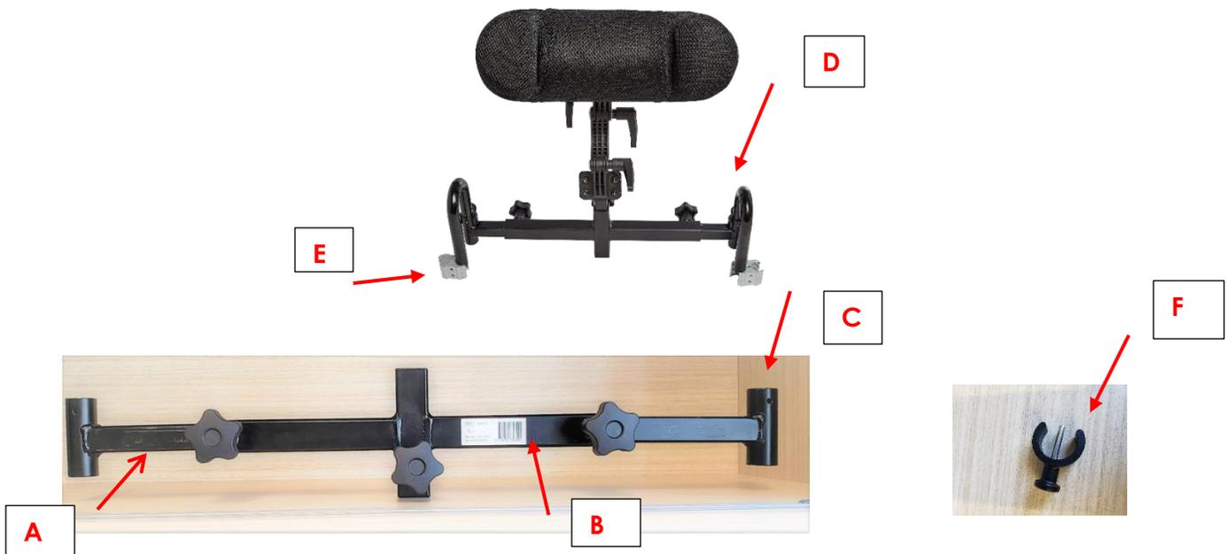
Insert telescoping side (A) into main bar (B). the knob of the main bar should be facing downwards and the hole on the round tube (C) should be facing you and upwards.
